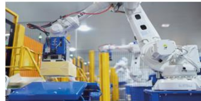
Robotic bulk cheese de-boxing unit
