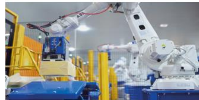
Robotic bulk cheese de-boxing unit
